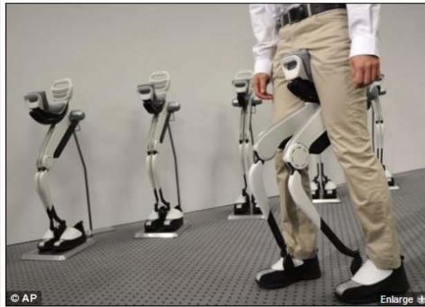
Ouch: Honda's latest assisted walking device looks like a bicycle seat connected by mechanical frames to a pair of shoes
